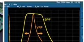
VRF Typical Bandpass Response (3.5 MHz)
