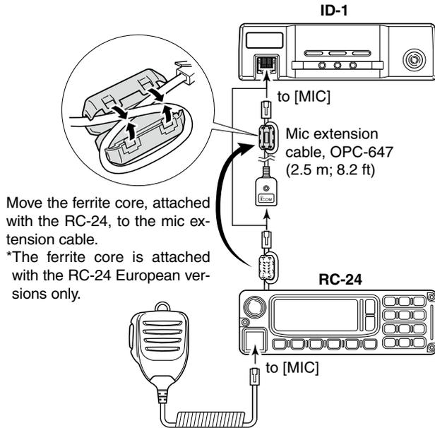
Move the ferrite core, attached with the RC-24, to the mic extension cable.
