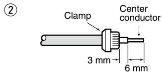
Strip the cable and fold the braid back over the clamp.
