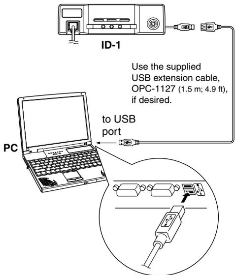
/// **NOTE:** When connecting the ID-1 and the PC through an USB hub, use the self-powered type.
