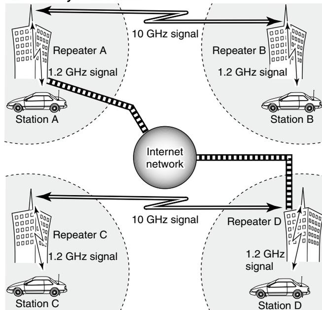
For current existing repeater operation, stations that are communicating must be in the same repeater's operating area. However, in the D-STAR system as in the illustration at left, the repeaters can be linked via the system repeaters (with a 10 GHz signal). Thus stations A and B can communicate even though they are in different repeater operating areas.
