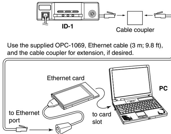
/// **NOTE:** When no Ethernet port is available with your PC, install an Ethernet card and its driver before connecting the ID-1. Ask your local computer dealer for details about installing a Ethernet card to your computer.
