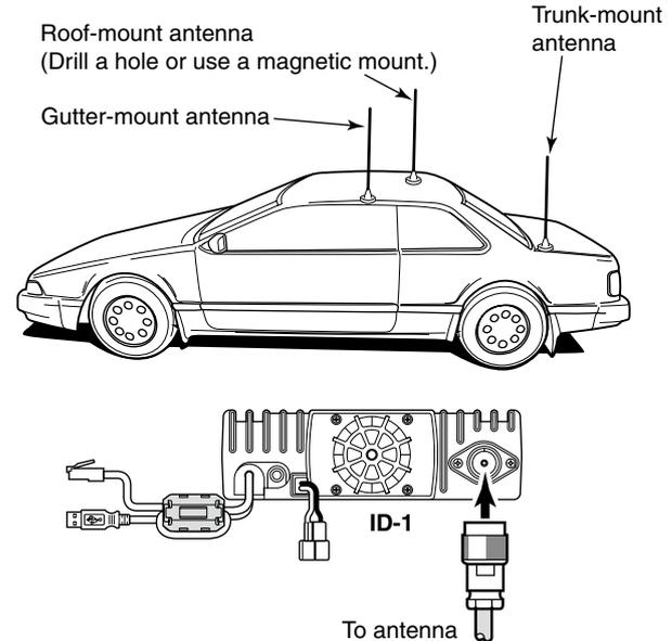
**Type-N CONNECTOR INSTALLATION EXAMPLE**
