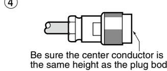
Carefully slide the plug body into place aligning the center conductor pin on the cable. Tighten the nut onto the plug body.
