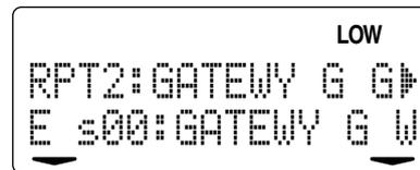
**NOTE:** When the near-by repeater is gateway repeater, push [∧] for 0.5 sec. (if necessary) after the call sign setting into "RPT1" in step ⑤ and skip step ⑥.
