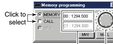
Shows the selected memory or call channel number and previously programmed frequency. Right click to move memory or call channel number up. Left click to move memory or call channel number down.
