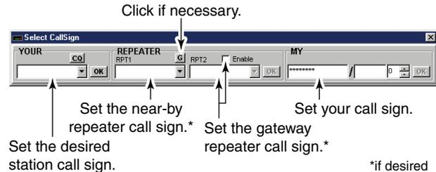
**NOTE:** When the near-by repeater is gateway repeater, set the call sign into “RPT1” then click [OK], and skip step ⑦.
