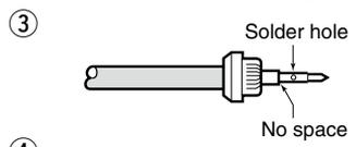
Soft solder the center conductor. Install the center conductor pin and solder it.
