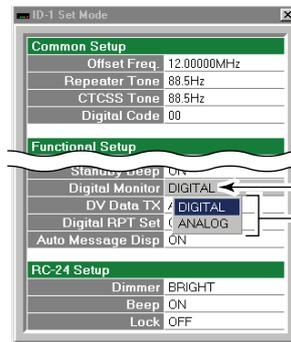
Double click the Digital Monitor cell, then select the desired monitoring mode.
