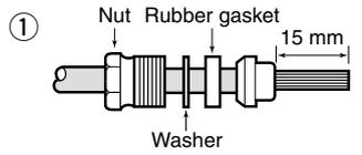
Slide the nut, washer, rubber gasket and clamp over the coaxial cable, then cut the end of the cable evenly.
